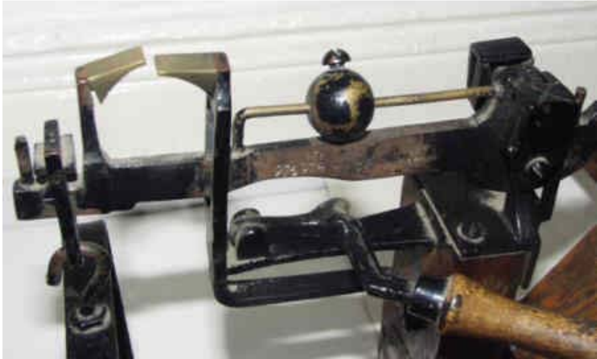
Detail of the balance indicators on platform scale
